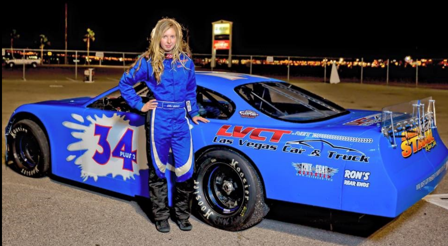
2014 Chevy SS NASCAR Super Late Model with a 350 Chevy small block on a Howe straight rail chassis built by Dana Stahl
